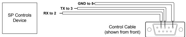
Connect male DB9 to projector port labeled *SERIAL IN*. *Serial Adapters* (for NRC only): A and B
